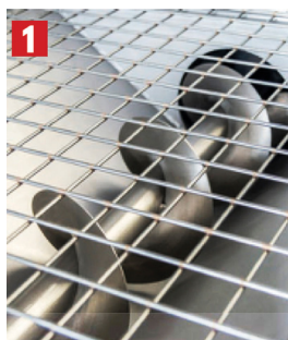
AISI 304 stainless steel feeding hopper with auger 1
