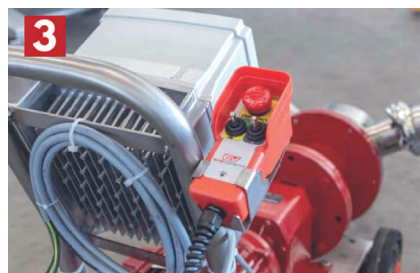
Electronic speed variator with remote cable control
