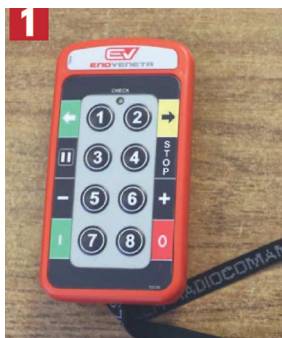
Electronic speed variator with remote radio control
